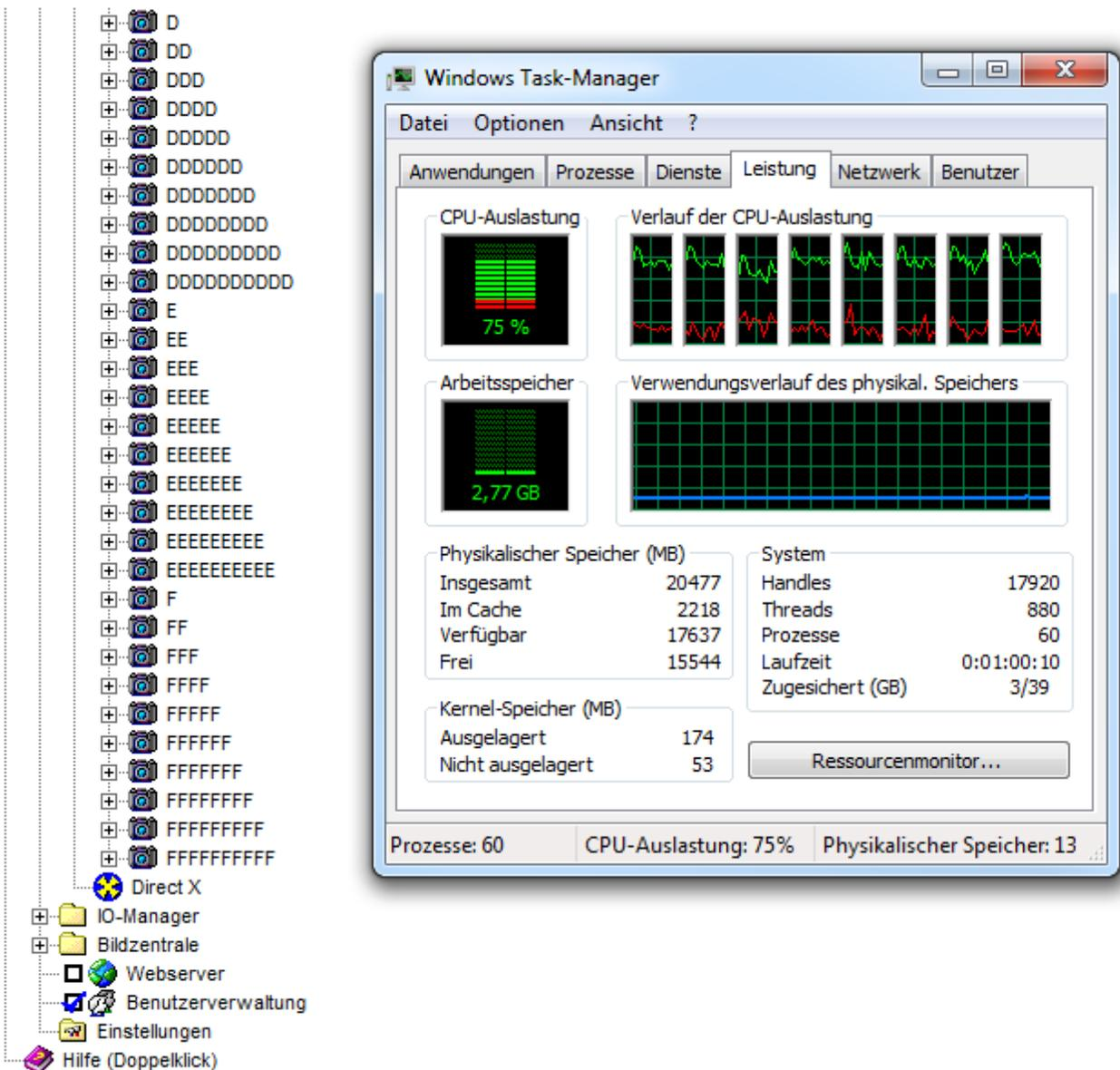
The **CPU load is 75%**, which means, in total, that an overall refresh rate of approx. **275 fps** is achieved.
