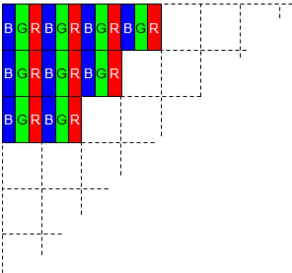
This means that each pixel consists of 3 bytes. As a result the size of an image with VGA resolution (640x480 pixels) is:
