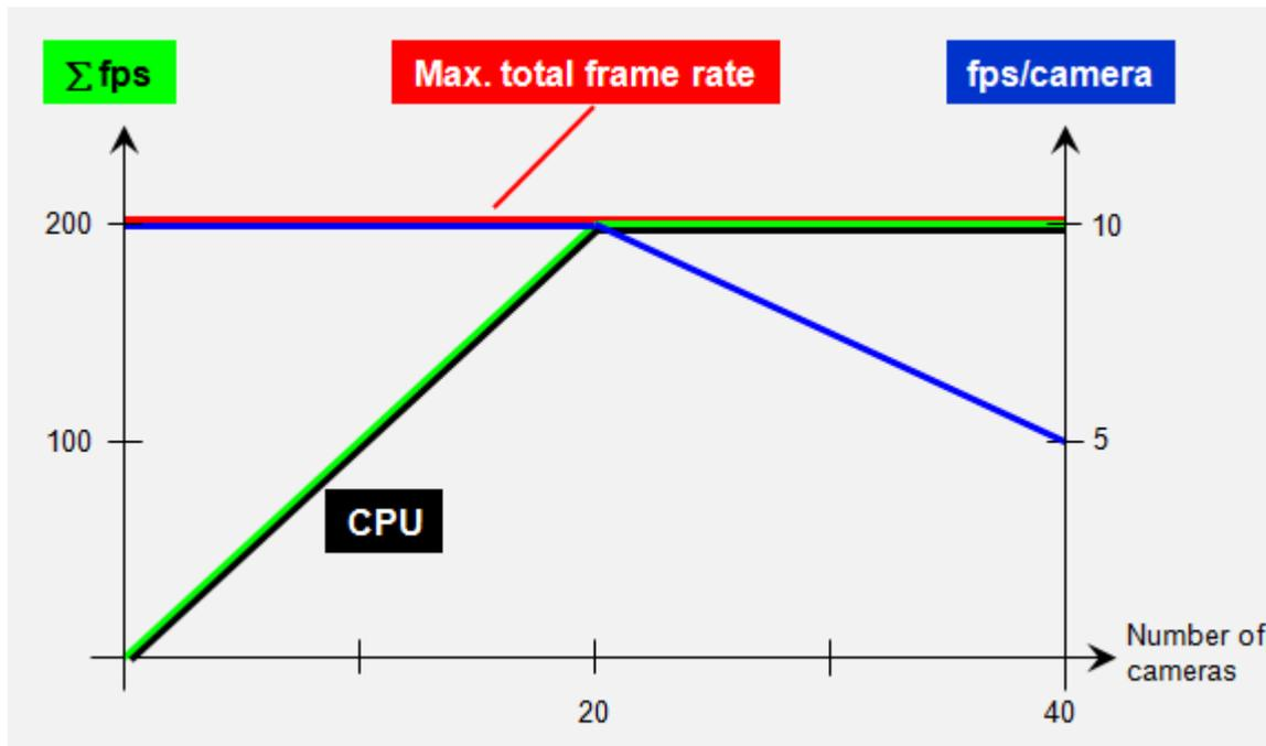
It is obvious that there is a linear increase in the CPU usage as the number of cameras grows, although the frame rate per camera remains the same (10 fps). With 20 cameras and a total of 200 fps, the PC is operating at full capacity. If more than 20 cameras are installed, the frame rate for each camera will decrease accordingly. With 40 cameras the maximum possible frame rate is only 5 fps per camera.
