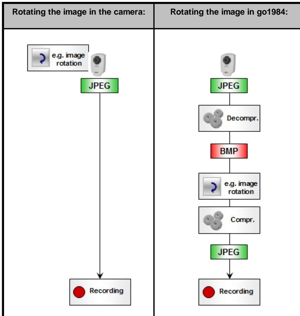
Click on the JPG button in go1984 to use the original image from the recording source (this is the default setting). Although it is no longer possible to edit the image, for example rotating, mirroring or adding a caption, this can almost always be done by the camera, which results in a significant improvement in the overall system performance.
